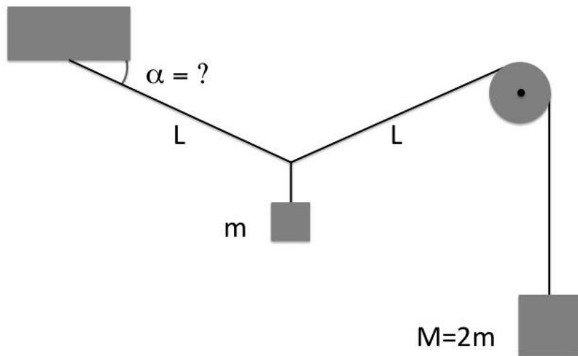
**Hint:** The sum of forces acting on each weight should be equal to zero in equilibrium. The tension of the rope on both sides of the pulley is the same.
