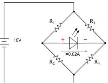
**Hint:** Assume that the voltage drop across LED and the current flowing through it are optimal: 2V and 0.02A respectively. Let current through resistor  $R_1$  be  $I_1$ . From here, find currents and voltages across other resistors.
